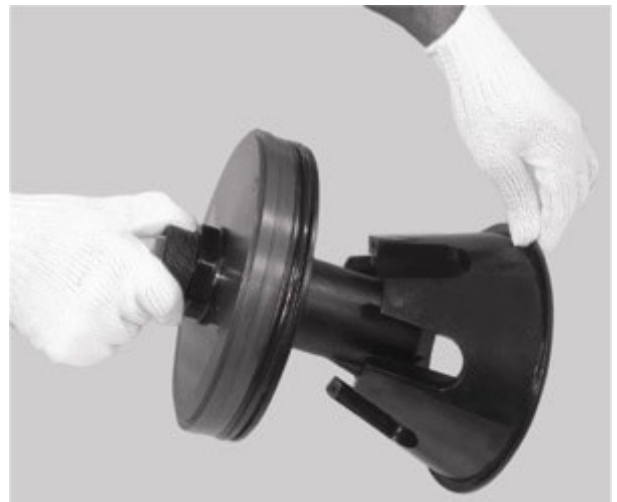
Installing Thrust Cone
