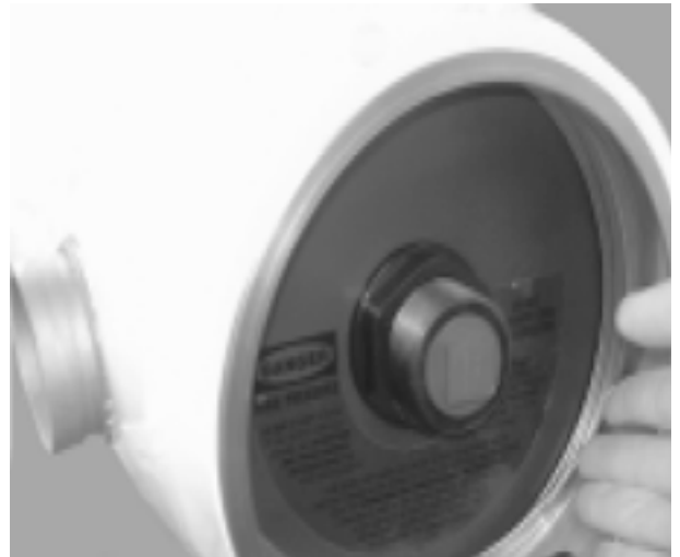
Installing Head Retaining ring
