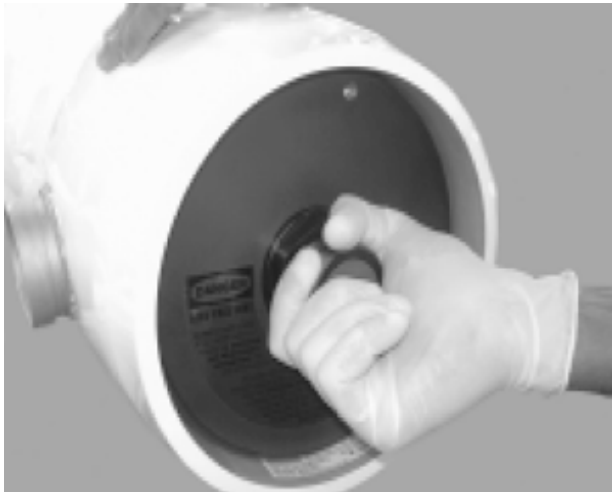
Installing Head Assembly
