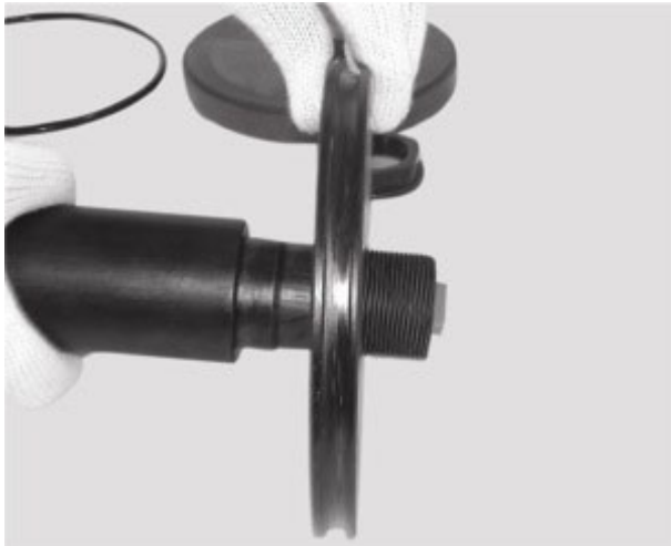
Installing Sealing Plate
