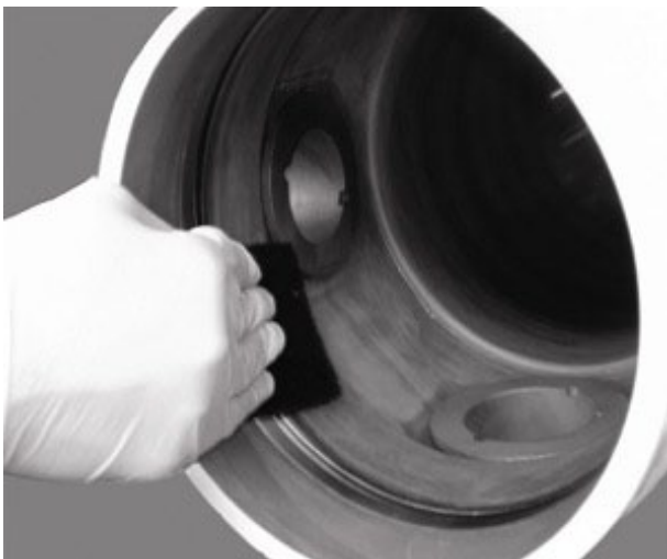
Cleaning inside the vessel
