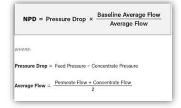
The Pressure Differential can help identify if the membrane is dirty. The normalized value (NPD) will account for changes in flow and temperature. An increase in the NPD is an early warning of scaling and/or fouling. To prevent complex problems the membrane should be cleaned if the NPD becomes 15% or greater than the baseline.
